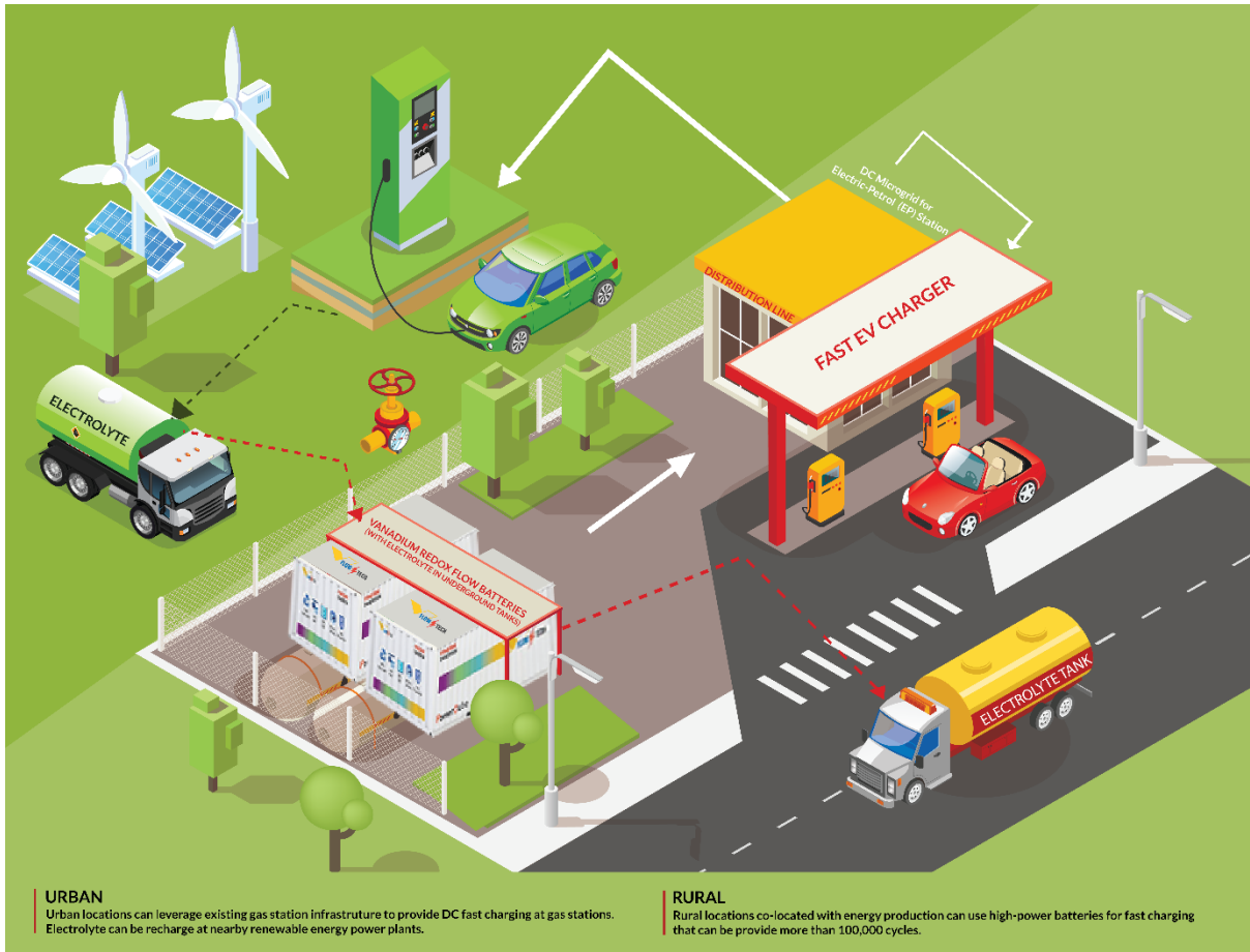
Schematic of a hybrid ESS supporting a smart urban micro-grid. (Link to download high-resolution image: Please click here )
