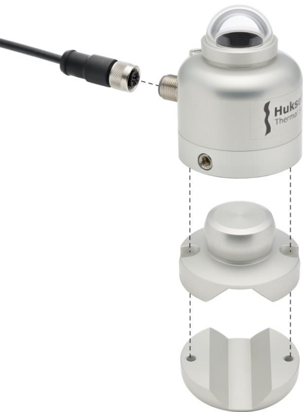
Figure 3 'Exploded view' of SR05. The optional ball levelling and tube mount allow for easy installation. The cable (standard 3 m) has an M12-A connector.
